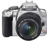
Digital SLR cameras will give you much more flexibility than compact cameras. The camera should have a Bulb, or B, setting, and allow you to manually adjust the focus, exposure, aperture, and film speed (or ISO).
